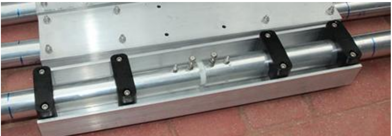
40M center sections mounted on element channels
