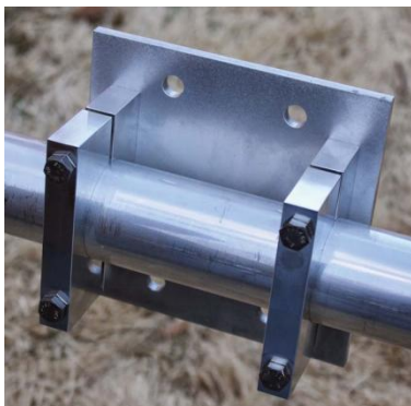
Boom to Mast Plate attached to Boom (Illustrative picture used)
