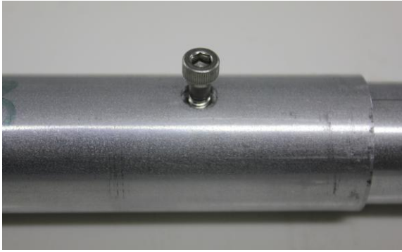
Screw fits into recessed hole - face up
