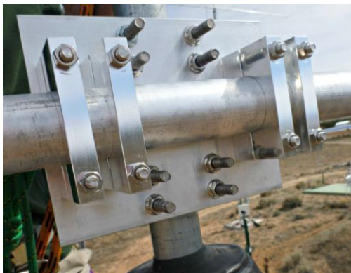
Boom to Mast Plate attached to Boom (Illustrative picture used)
