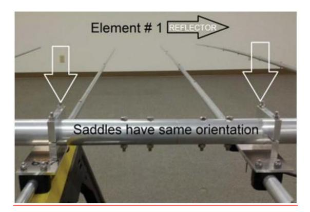
Before final torquing, re-check spacing and horizontal alignments of element center sections on the boom using the measurements illustrated on Diagram 1.
