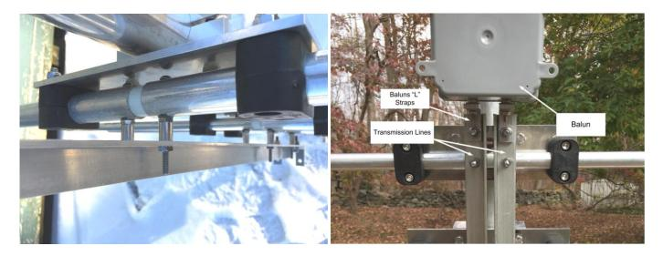
The JK NAVASSA-5 is delivered without a balun. We recommend a 1:1 current balun since the antenna is designed to be fed with a 50 Ohm balanced source, bringing the antenna to true optimum performance.
