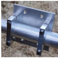
Boom to Mast Plate attached to Boom
