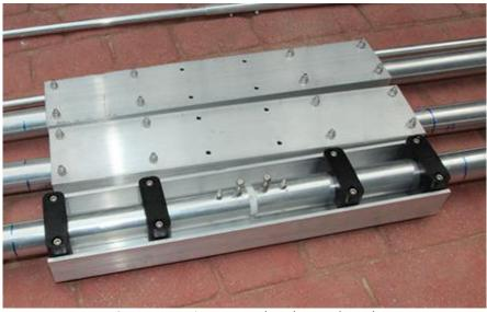
40M center sections mounted on element channels
