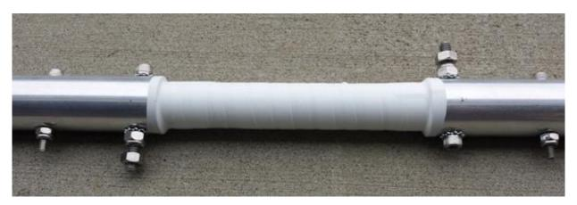
10) Slide the coil onto the assembly; thread the 10-24 screw four to five times directly into the coil standoff.
