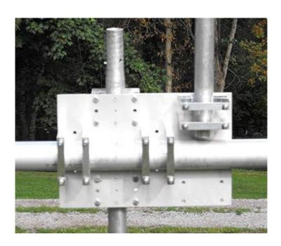
Boom/Mast plate mounted on temporary mast (for illustrative purposes only - this configuration not valid for all antennas)
