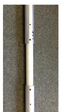
The fiberglass rod has 4 holes, two of which are 1/4" holes, and two of which are #10. The #10 holes are the outside holes from the center and are used for the mechanical mounting of the tubing to the fiberglass. The 1/4" holes are used for mounting the coil.
