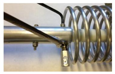
NOTE: It is very important to have a solid mechanical connection, with the nut and screw making a tight contact over the tubing. Visually inspect the coil assembly for any twists or non-symmetry while tightening these nuts. Adjust them carefully by pulling them back into place. Repeat this same process for all the coil assemblies.
